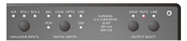
With the "ANALOGUE INPUTS" and "DIGITAL INPUTS" buttons on the front of VIOLECTRIC DHA V590² one of three analogue inputs or one of four digital inputs may be activated. The corresponding LED is illuminated. Concerning the digital inputs, also the "PCM" or "DSD" LED is on as long as an appropriate digital signal was detected. When there is no signal on these inputs or a non-valid signal, these LEDs will stay dark and the outputs are muted.
